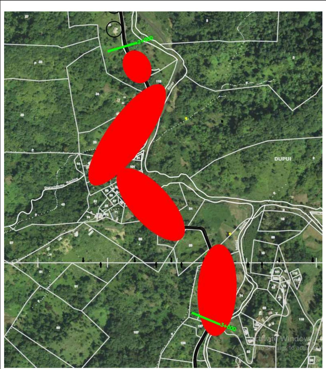
Figure 57 Zone A (human impact) receptors between chainage 2 km and 3 km classified as Zone 3 in impact severity.
