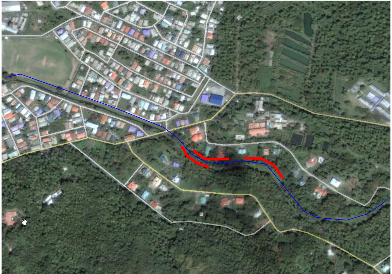
Figure 36 : Embankment protections localization
