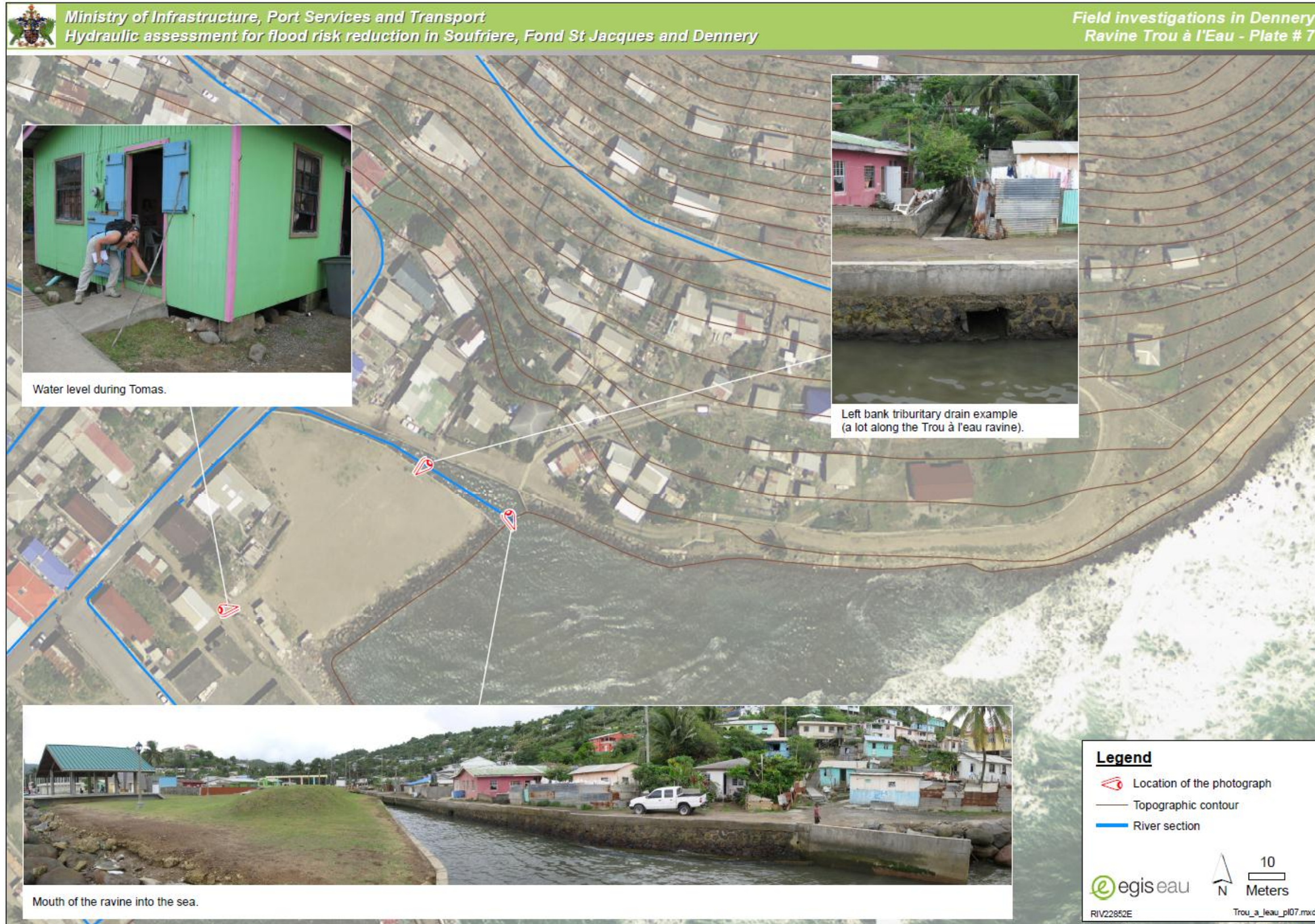
Figure 19 : Field Investigation in Dennerly : Ravine Trou à l'Eau – Plate # 7
