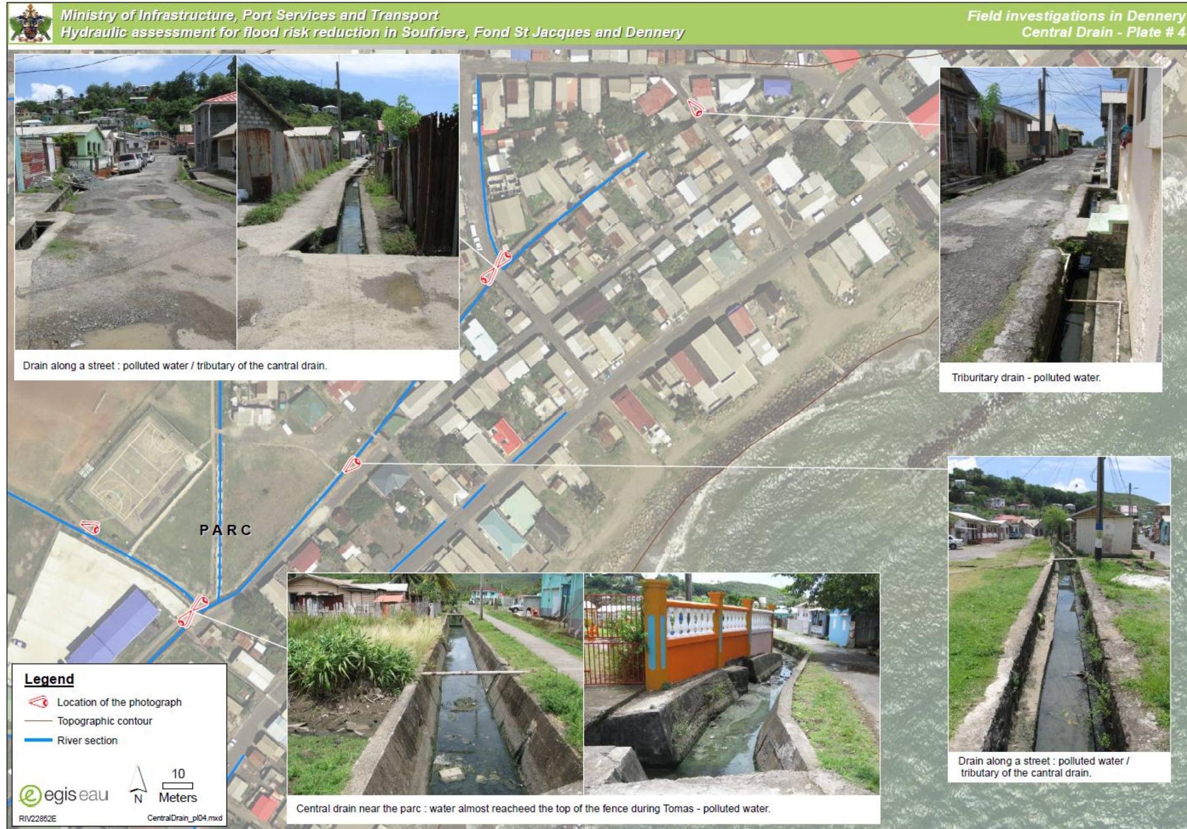
Figure 24 : Field Investigation in Dennerly : Central drain – Plate # 4
