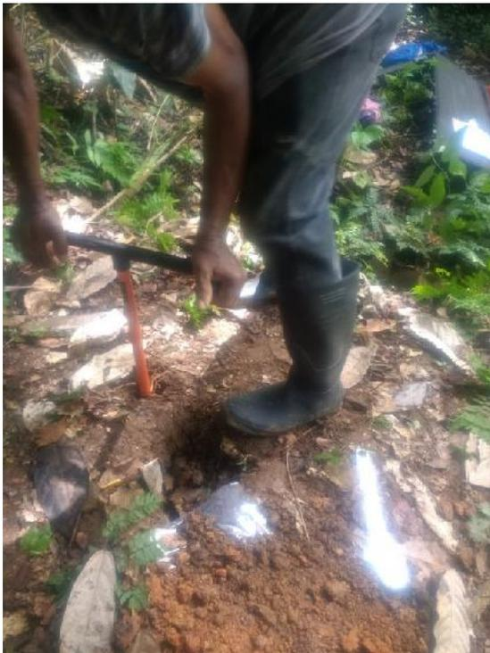
*Photo 3: Auger Sampling along piperoute*
