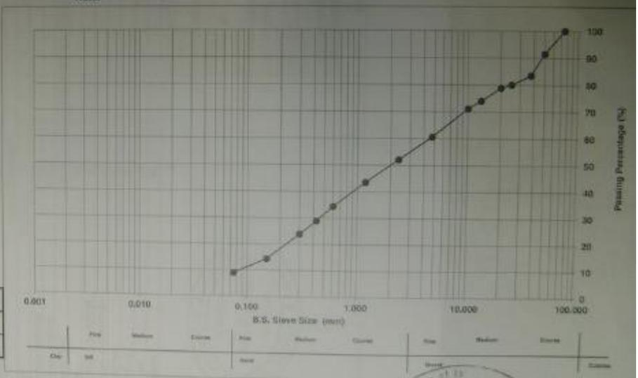
**Figure 14** showing Sieve Analysis for Fill from Millet Quarry
