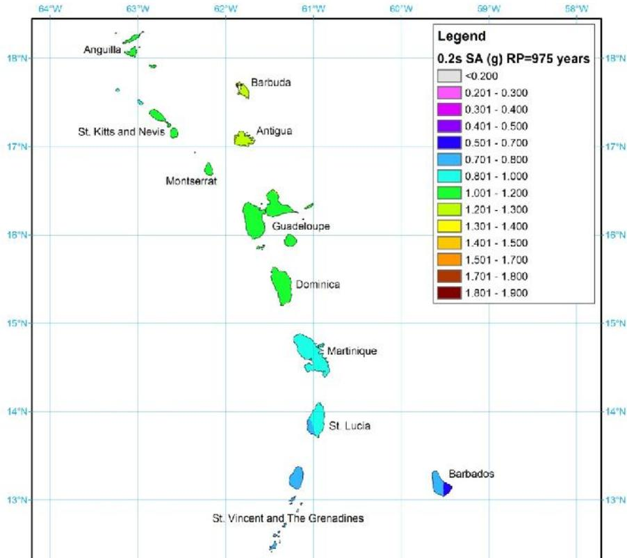
**Figure 8:** Seismic Hazard Map for 0.2s Acceleration and return period of 975 years
