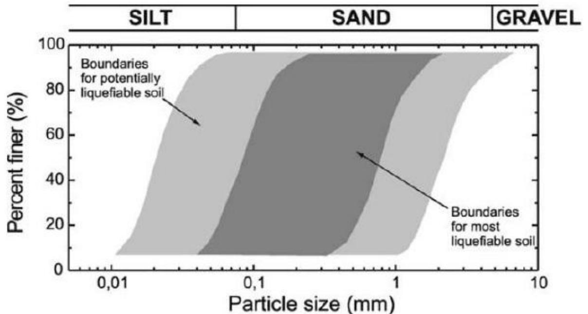
**Figure 9:** *Grain Size of liquefiable soil (Tsuchida 1970)*
