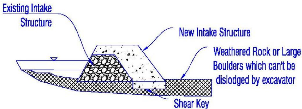
**Figure 11** showing section of proposed new intake structure integrated into existing
