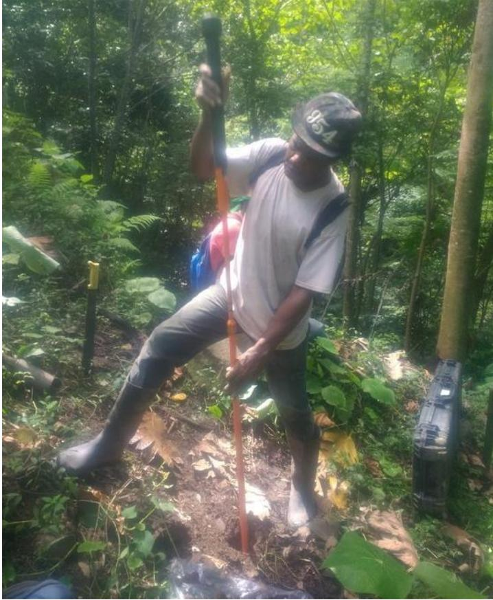
*Photo 6: Undisturbed Sampler with Hammer*
