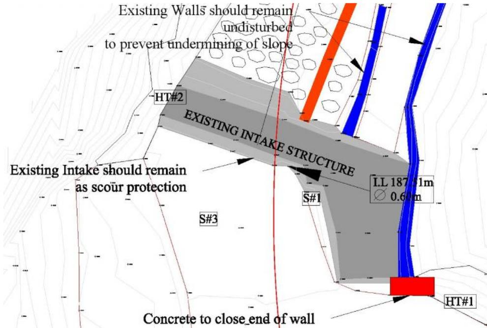
**Figure 10** showing recommendations for existing intake structure.
