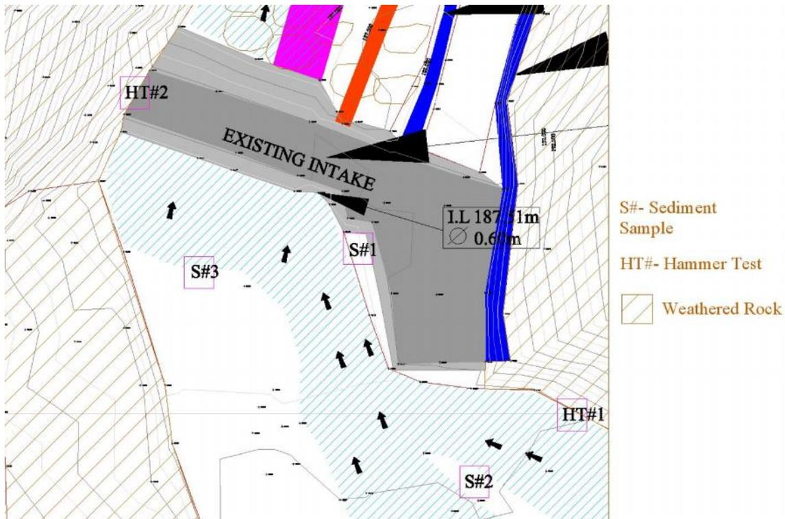
**Figure 5: Location of soil samples and hammer tests**
