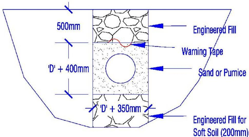
**Figure 12** showing typical pipeline trench
