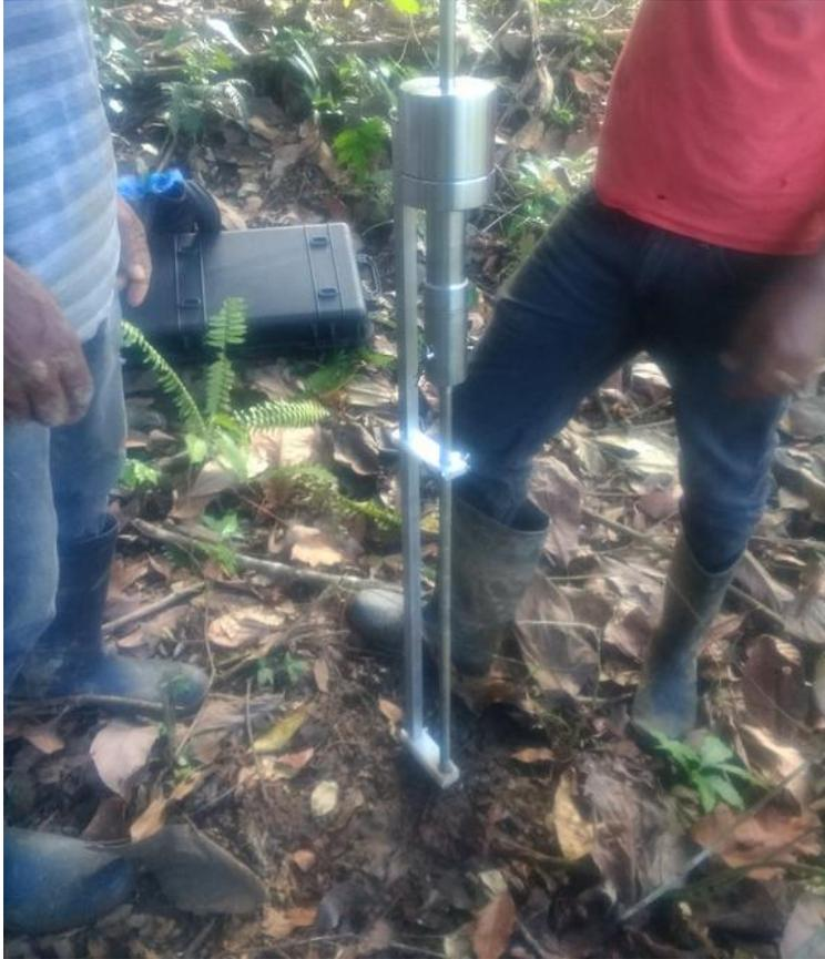
*Photo 4:DCP Testing along Piperoute*
